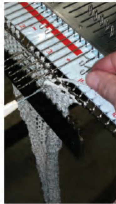
STEP 2 KNIT PIECE KEEP PROPERLY WEIGHTED FOR TENSION CONSISTENCY WASH PIECE
