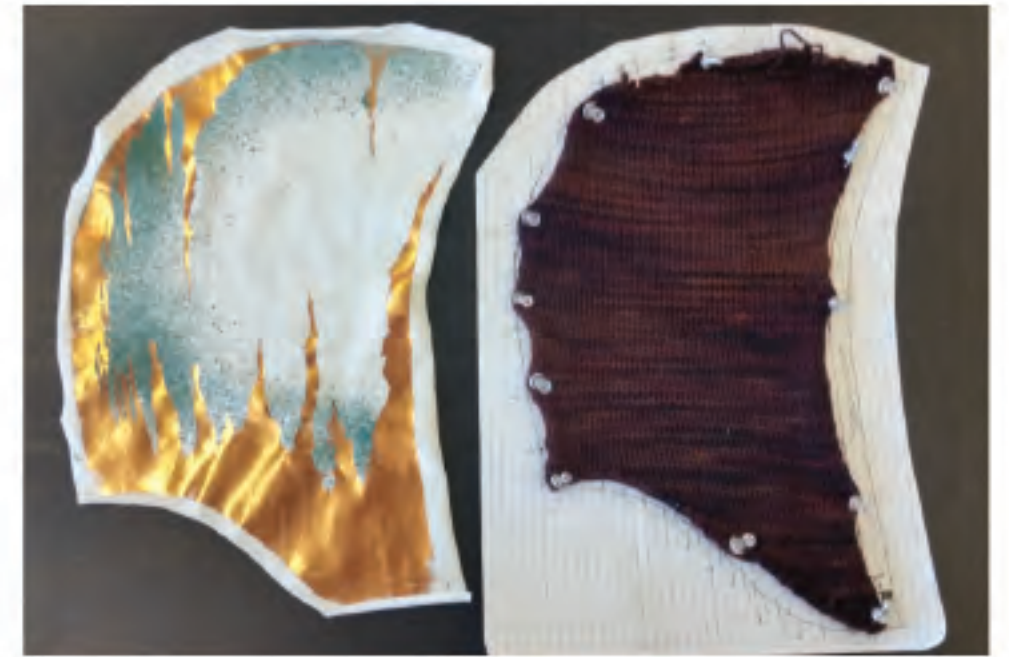
STEP 5 DIVIDE OUT LAYERS AND PRINT INITAL PRINT TESTS WERE DONE ON STANDARD KNIT JERSEY BEFORE APPLIED ONTO FULLY FASHIONED KNITTED PIECES.
