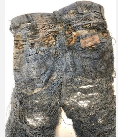
Figure 3: Biodegraded Wrangler Jeans with just Synthetics Left After 20 Years, by Sean Gormley
