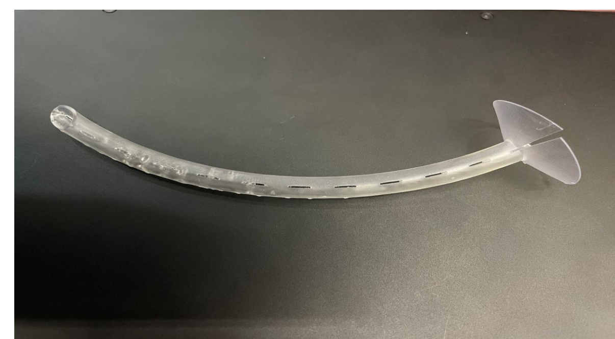
Prototype 2: 3D printed Flexible Material on Stereolithography printer
