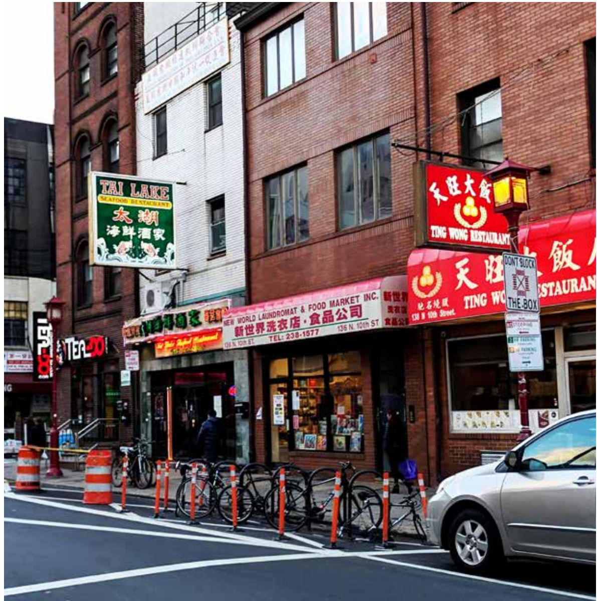
The bicycle corral in Chinatown takes up one parking space in the right-of-way while providing much needed space off the sidewalk for bike parking. (Photo by The Lindy Institute, 2018)
