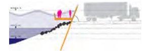
Perimeter protection of Hunts Point Waste Water Treatment Plant allows barge service transfers and maintains operability of the plant during storms
