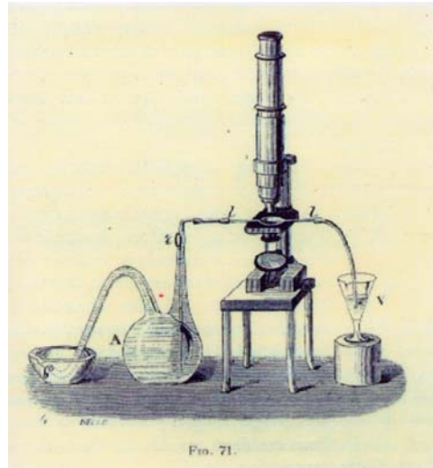
Figure 2. (a) Geissler Chamber; These chambers are flattened glass tubing that allow for culture liquids to pass slowly through, perhaps influencing the development of the microorganisms living in the chambers, (b) Geissler Chamber with a microscope. [Louis Pasteur, Études sur le vinaigre: sa fabrication, ses maladies, moyens de les prévenir: nouvelles observations sur la conservation des vins par la chaleur [Paris: Gauthier-Villars V. Masson et fils, 1868]]
