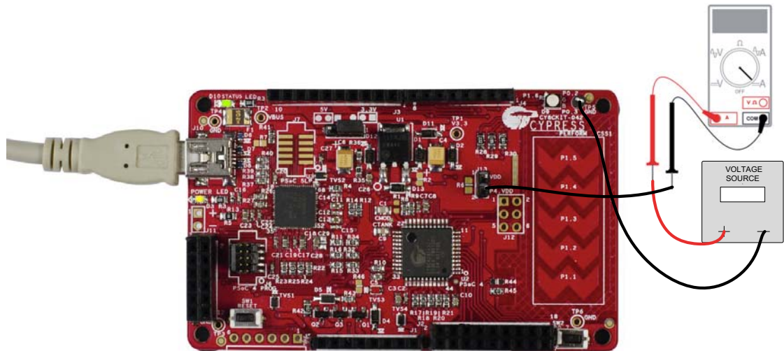
Figure 4-6. PSoC 4 Current Measurement when Powered Separately
