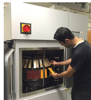
PhD student, Siavash Vahidi tests samples inside a xenon weatherometer
