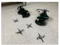
This project aims to develop a multi-robot target tracking system and design coordination algorithms for the robots (drones) to actively track dynamic targets (ground robots).
