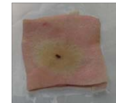
High dose rate (14J/s) – causes burns on the skin (5sec treatment, 70J total)
