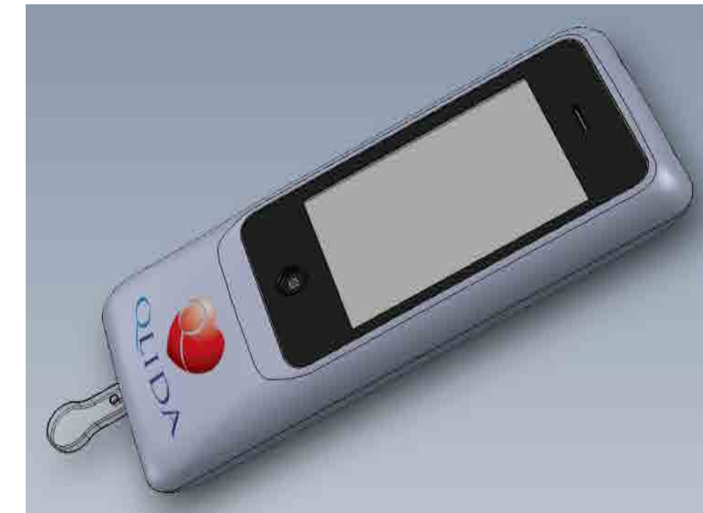
Handheld concept: Exploit built-in power of smart phone with simple, miniaturized reader concept
