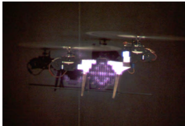
NRL dual-rotor UAV with PV array, illuminated with fiber laser during power beaming flight tests in LASR facility (2013).
