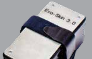
The Exo-Skin, a robotic glove developed at Drexel to help restore function to people with hand injuries
