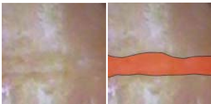
An ordinary image of a thermally damaged chicken skin tissue sample taken with an ordinary CCD camera (left) and a dielectric contrast image (right) recorded using our technique
