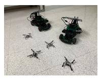
This project aims to develop a multi-robot target tracking system and design coordination algorithms for the robots (drones) to actively track dynamic targets (ground robots).
